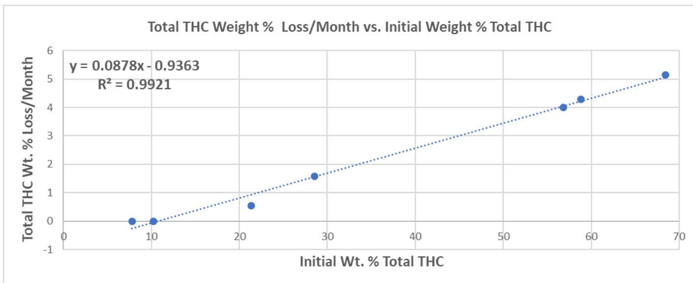
**Figure 2** A plot of total THC degradation rate versus initial total THC concentration for a collection of 7 cannabis extract samples.
