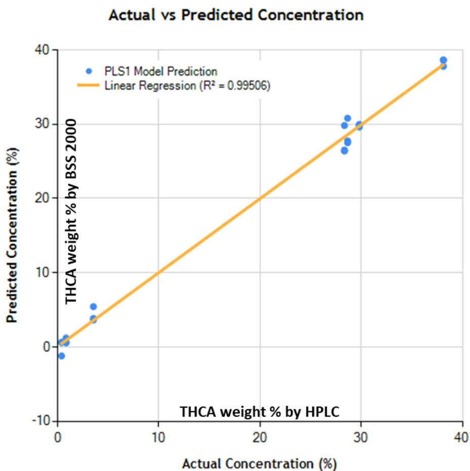
**Figure 2** Plot of weight percent total THCA in cannabis oils as determined by HPLC versus as predicted for the same samples by the BSS 2000 Cannabis Analyzer. Note the correlation coefficient of 0.995.
