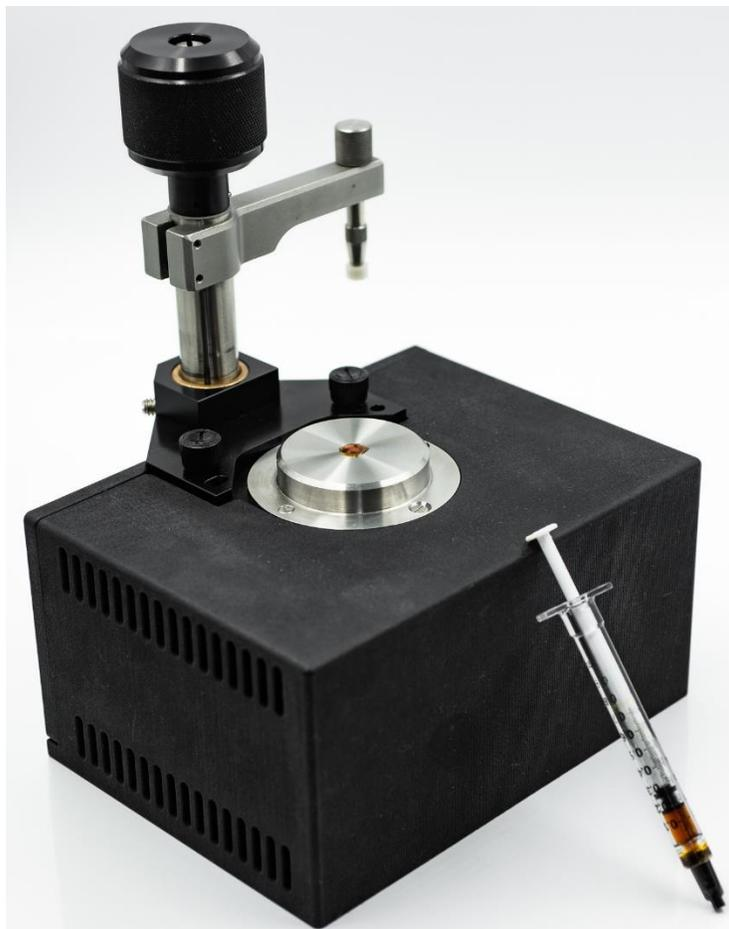
**Figure 1** A photo of the BSS 2000 Cannabis Analyzer with a sample of cannabis oil resting on its sampling window.
